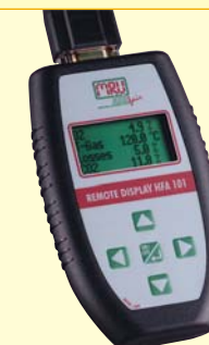
Handheld remote control incl. 10 (20) m transmission cable
